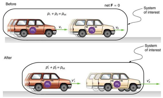
Figure 8.3 A car of mass  $m_1$  moving with a velocity of  $v_1$  bumps into another car of mass  $m_2$  and velocity  $v_2$  that it is following. As a result, the first car slows down to a velocity of  $v_1'$  and the second speeds up to a velocity of  $v_2'$ . The momentum of each car is changed, but the total momentum  $p_{tot}$  of the two cars is the same before and after the collision (if you assume friction is negligible).
