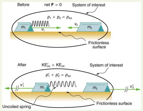
Figure 8.10 An air track is nearly frictionless, so that momentum is conserved. Motion is one-dimensional. In this collision, examined in Example 8.6, the potential energy of a compressed spring is released during the collision and is converted to internal kinetic energy.
