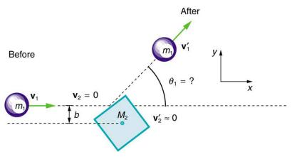
Figure 8.16 A small object approaches a collision with a much more massive cube, after which its velocity has the direction  $\theta_1$ . The angles at which the small object can be scattered are determined by the shape of the object it strikes and the impact parameter  $\,b\,$  .
